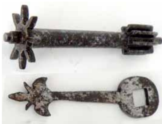
Fig. 7. The hand and the 8-tooth right-angle starwheel drive to the countwheel.
