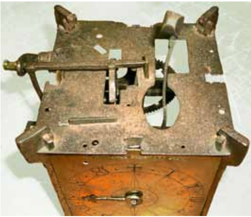
Fig. 6. Top view showing the wedges holding the pillars to the top plate and the later anchor escapement. Empty holes indicate the location of the removed balance-wheel cock, frets and side doors. Note the broken horizontal hammer stop.
