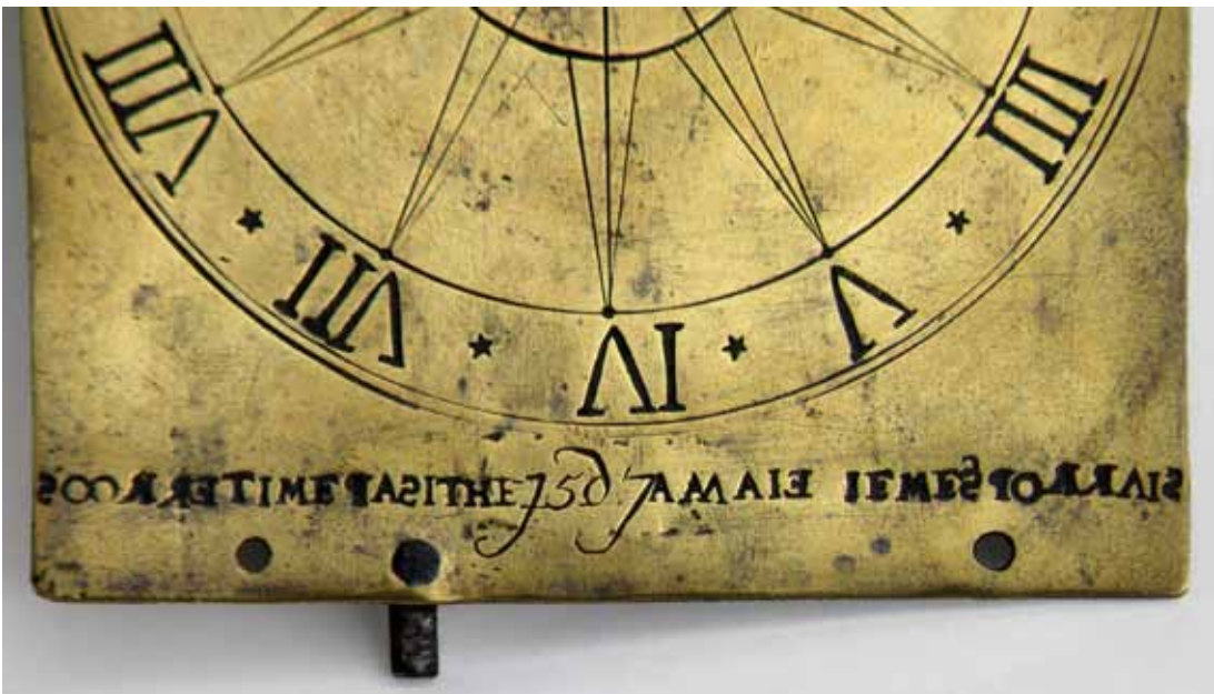
Figs 14 & 15 Details of the punched inscriptions, the punched chapter ring and the engraved date 1567.
