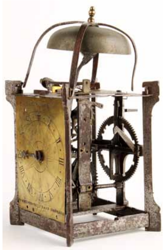
Fig. 3. Right-hand side showing the drive to the countwheel. The starwheel of the similar drive to the dial wheel is just visible.
