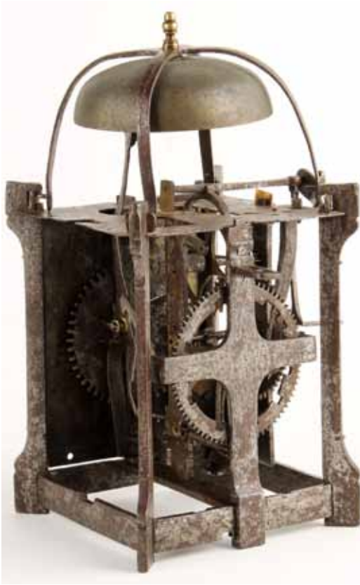
Fig. 4. Rear view showing the countwheel with internal slots mounted inside the rear cruciform movement bar.
