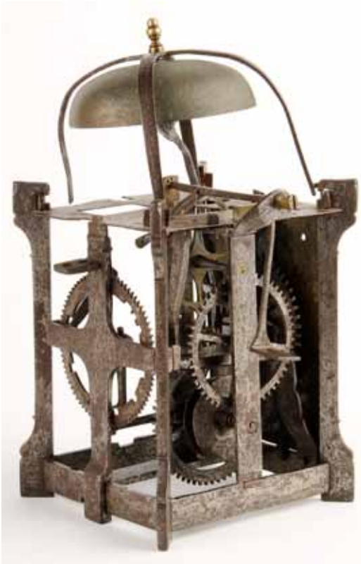
Fig. 2. Left-hand side showing the wheels of the going train at right angles to the dial, with the countwheel at the rear. Note the later escapewheel and pendulum crutch.
