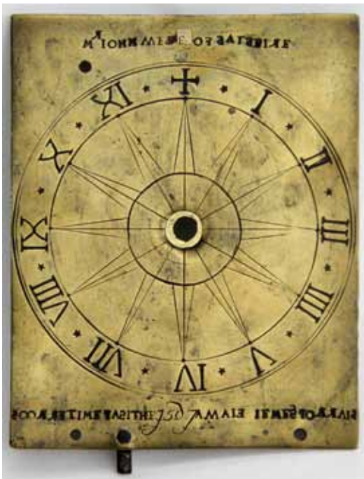
Fig. 12. The dial showing the central bush to compensate for the removed alarm.
