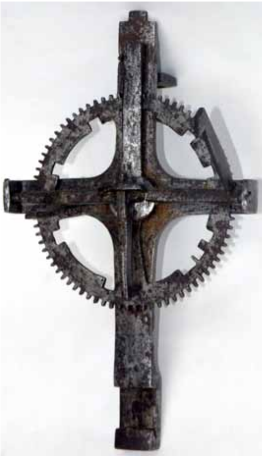
Fig. 8. Rear movement bar with the countwheel pivoted on the inner face and the locking arbor pivoted between the end returns. The countwheel detent hangs down from the centre, the locking detent points upwards on the right, while the arm that once held the nag's head is on the left. Note the dovetailed hook at the bottom.
