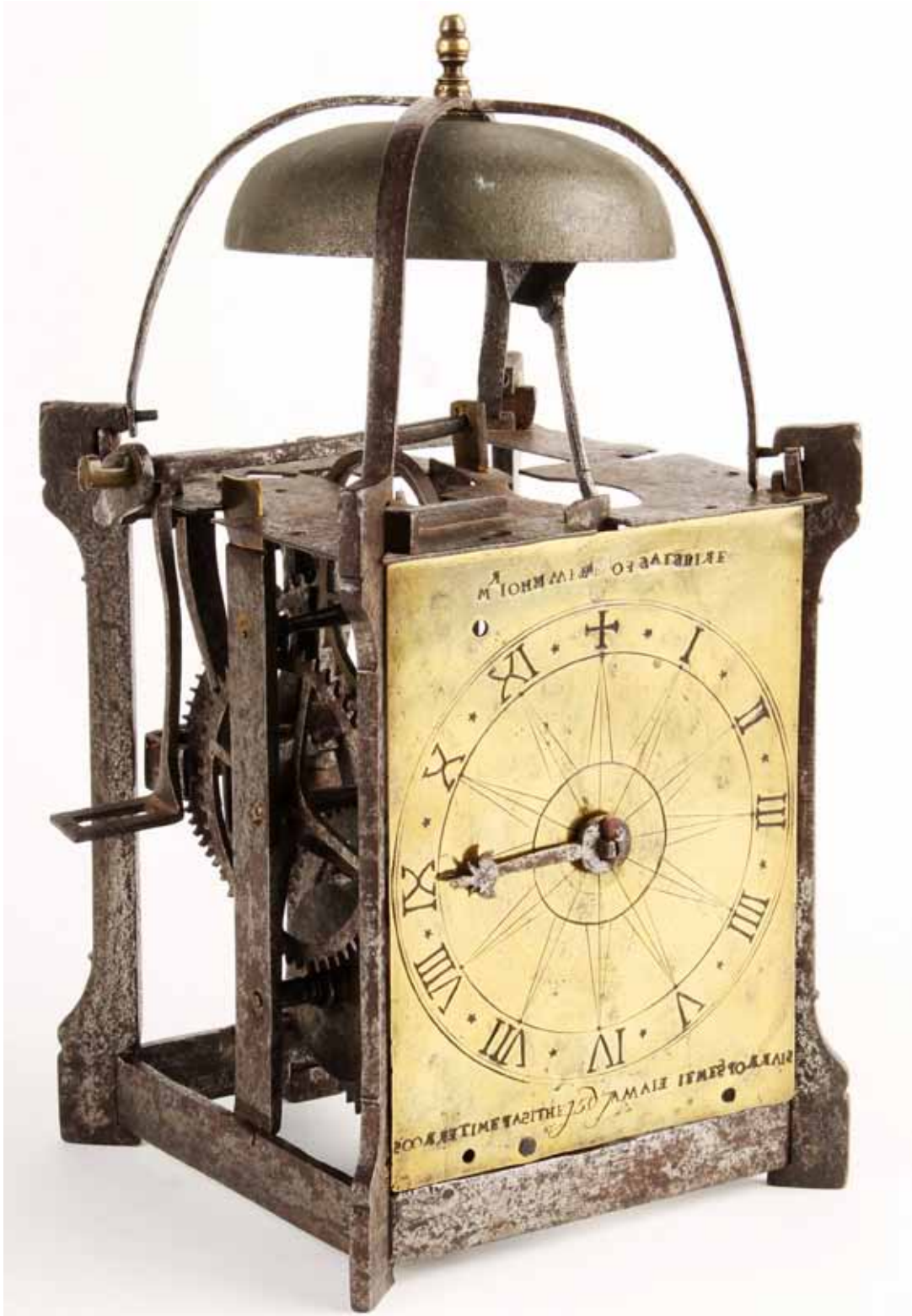
Fig. 1. Front view of the Porrviss clock with the later pendulum escapement on the left-hand side. The bell and finial are probably later.
