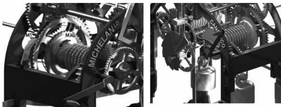
Figure 3. Left and right views of the charging mechanism of the Canonico's clock in a virtual reconstruction.
